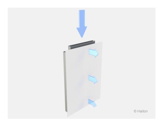
Air is supplied into the space through the front panel of Halton Zen Rectangular in Wall, generally at a slightly lower temperature than the room air. The supply airflows down to the floor level, before gradually pervading the occupied zone at a low velocity. Finally the convection of warm surfaces causes the air to rise out of the occupied zone. The low velocity flow pattern is directed forwards.
