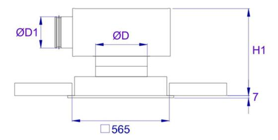
The collar of the Halton TRI plenum can be installed either internally in the plenum or externally onto the bottom of the plenum. The height of the unit is presented in the table below for the external installation. When the collar sleeve is installed internally, the total height H is reduced by 60 mm.
