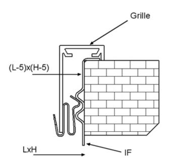
The grilles are supplied with clips fastening as standard with the IF installation frame.
