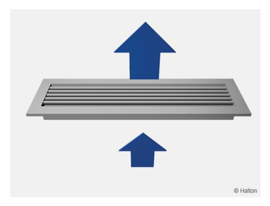
Supply air is supplied without deflection through the horizontal vanes into the space. Supply air mixes with room air in front of the grille.
