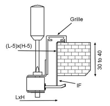
Concealed screw fastening is possible when the grille is installed with an installation frame (IF).
