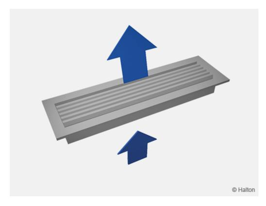
Supply air is supplied with a 15° angle deflection through the horisontal vanes into the space. Supply air mixes with room air in front of the grille.
