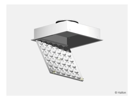
Detach the front panel of the diffuser by gently pulling it down and let it balance on the hinges. Each nozzle can be easily removed by pressing the stoppers and then pushing the nozzle through the front panel.
