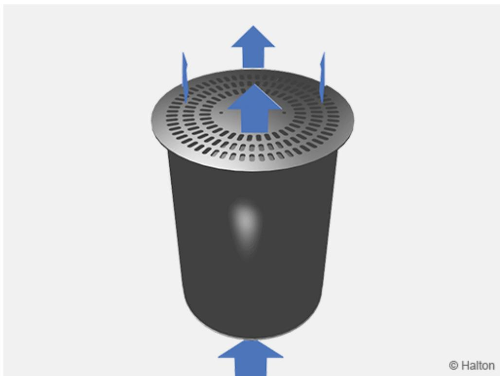
Halton BCF floor diffusers are designed for under-floor air distribution systems. Air is supplied into the space through the front panel at a low velocity, mixing with room air above the diffuser. The perforated plate inside the plenum box creates sufficient pressure loss to enable self-balancing.
